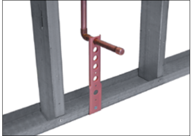
Figure 12-10 Poor Attempt at Dissimilar Metal Isolation
